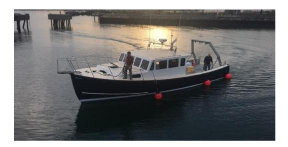
Our 46' Survey Vessel *R/V Galatea* is the newest addition to Semper Diving and Marine's offshore capabilities. *Galatea* has undergone extensive upgrades over the past year to accommodate for surveying, diving, and robotics work. She is equipped with spacious available lab space, a heavy duty hydraulic A-frame and winch, ample deck space, sub-meter resolution survey quality GPS, and more. Click below for *Galatea*'s complete informational brochure.
